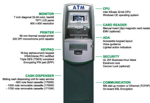
Figure 1: An example of ATM and its modules (Model: Hantel 1700)
