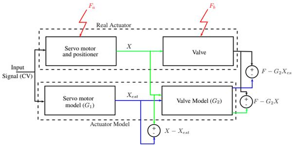
Figure 5: Structured residuals block diagram
