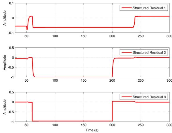
Figure 9: Residuals for the valve with fault  $f_3(f_d = -1)$
