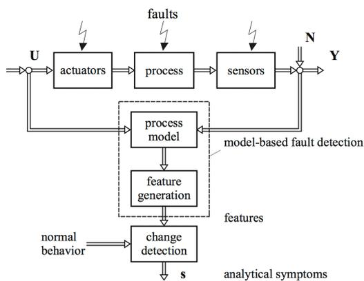
Figure 1: Model based fault detection method
