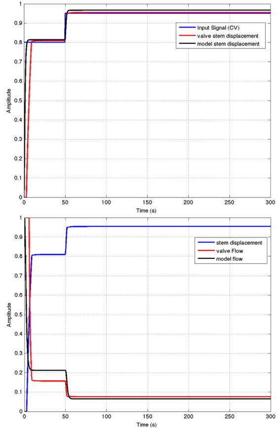
Figure 4: Step responses of valve and model
