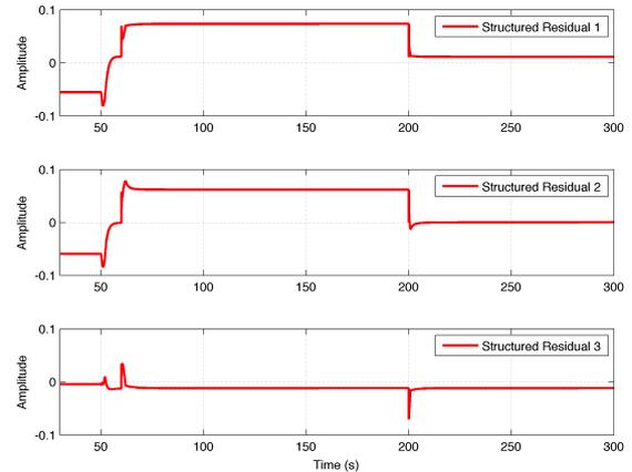
Figure 8: Residuals for the valve with fault  $f_3$
