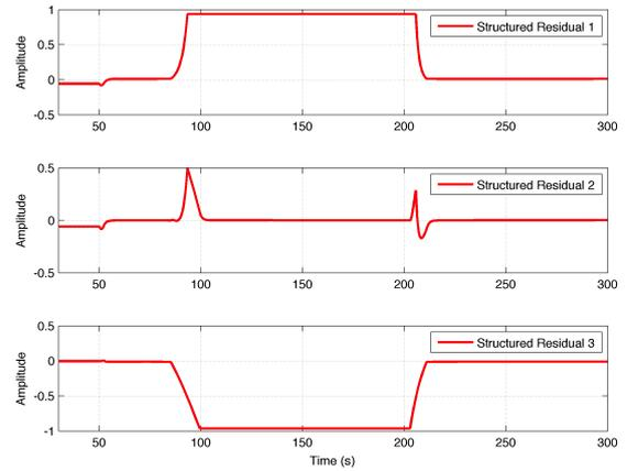
Figure 7: Residuals for the valve with fault  $f_{16}$
